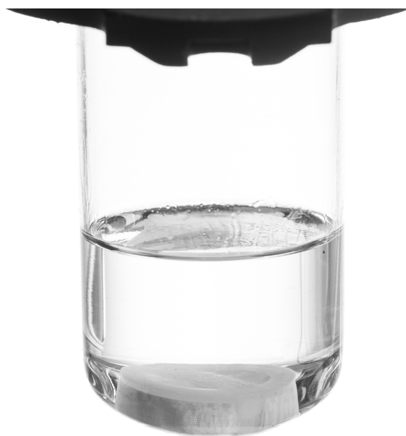
Figure 1. A SpinChem® MagRBR filled with Reaxa Pd(II) EnCat TPP30 in an EasyMax™ 102 Advanced synthesis glass vessel.
