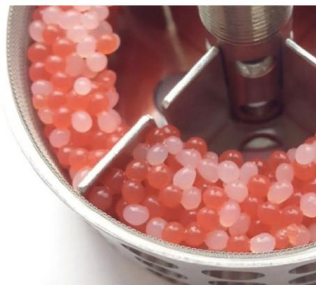
Efficient synthesis of chiral lactones by encapsulated cells in a rotating bed reactor.
