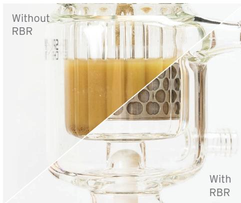
Rotating bed reactors completely avoid grinding of molecular sieves.
