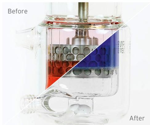
Effective phase-transfer between immiscible liquids and an ion exchange resin.
