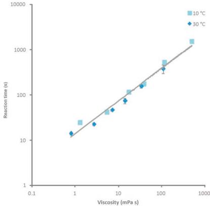
Consequences of viscous solutions on the reaction rate with rotating bed reactors.
