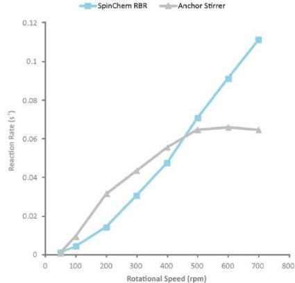
Optimizing the rotational speed of rotating bed reactors in baffled reaction vessels.
