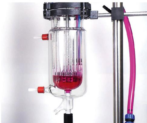
Automated semi-continuous batch processing system with rotating bed reactor.
