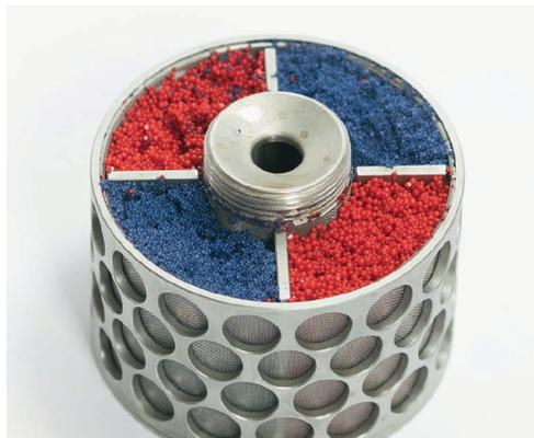
Simultaneous extraction of two dyes selectively onto different resins.
