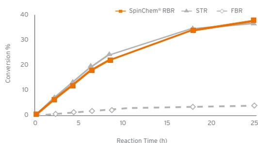
**Fig 3. Formation of  $\epsilon$ -caprolactone by CHMO enzyme inside calcium-alginate encapsulated *E. coli* cells (28 g wet) using either SpinChem® RBR, STR or FBR reactor setups. Conditions: cyclohexanone (20 mM) and D-glucose monohydrate (2.5 g/L) in 0.5 L Tris-HCl buffer (20 mM, pH 7.5, 1% NaCl). Vessel setup cf. Fig 2. FBR flow 3 mL/min.**
