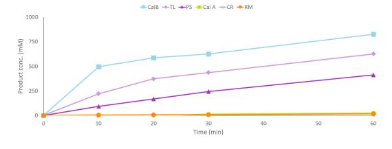
Figure 3. Formation of propyl laurate over time for esterification reactions catalysed by different immobilized lipases.
