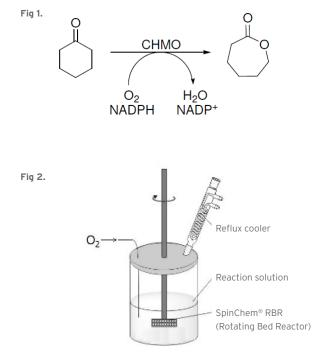
Fig 1. Synthesis scheme for production of  $\epsilon$ -caprolactone from cyclohexanone by cyclohexanone monooxygenase (CHMO).
