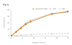
Fig 3. Formation of ∂-caprolactone by CHMO enzyme inside calcium-alginate encapsulated *E. coli* cells (28 g wet) using either SpinChem<sup>®</sup> RBR, STR or FBR reactor setups. Conditions: cyclohexanone (20 mM) and D-glucose monohydrate (2.5 g/L) in 0.5 L Tris-HCl buffer (20 mM, pH 7.5, 1% NaCl). Vessel setup cf. Fig 2. FBR flow 3 mL/min.
