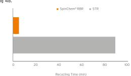
Fig 4. Remaining activity (a) of calcium-alginate encapsulated *E. coli* cells with CHMO after recycling to consecutive batches. Total time for recycling (b). Two hours reaction time for each batch. Conditions cf. Fig 3 plus 20 mM CaCl<sub>2</sub>.
