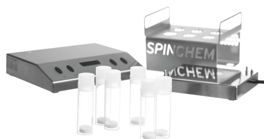
Fig 1. SpinChem® MagRBR starter kit, including six MagRBRs pre-packed with resin, reaction tubes, six-position magnetic stirrer, stirrer control unit and tube rack.
