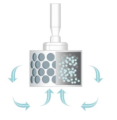
The SpinChem® RBR creates efficient mass transfer. The RBR aspirates solution from the bottom, percolates it through the bed of solid phase, and finally distributes it towards the vessel wall, thereby creating a continuous flow of solution.
