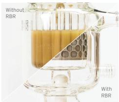
Effective phase-transfer between immiscible liquids and an ion exchange resin.
